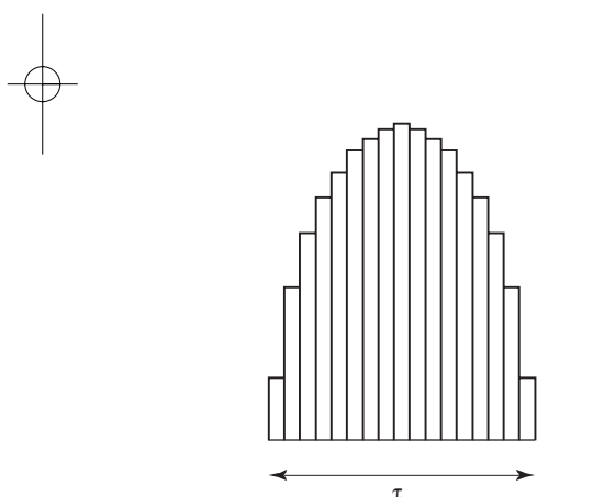
Figure 9.17 A selective pulse can be divided into small elements (points), with the minimum length of each element determined by the spectrometer hardware. The sum of the elements ( \tau ) is the total length of the pulse. To achieve off-resonance excitation, each element will have a phase increment ( \theta ) determined as in Equation 9.10.
